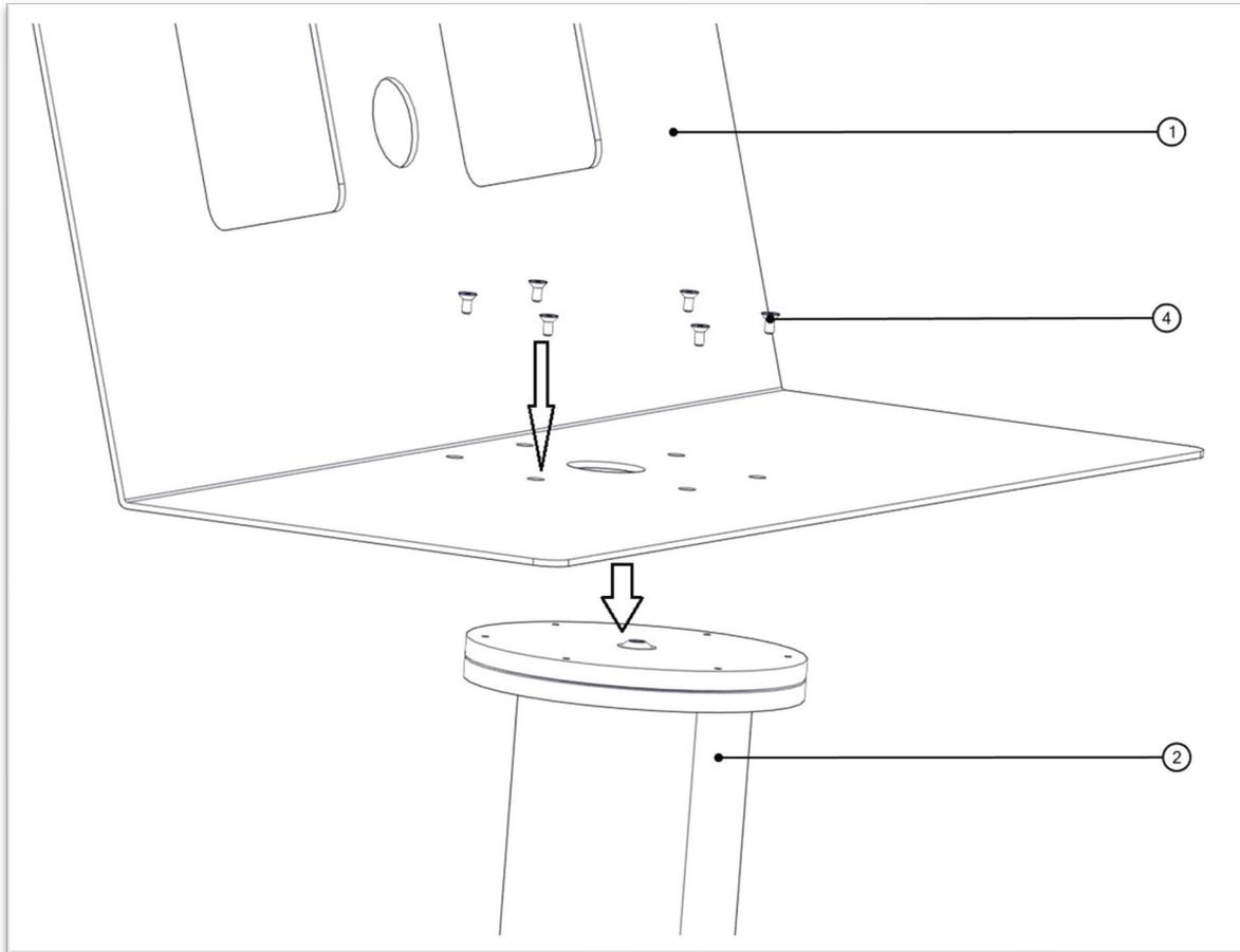
**Figure 5: Attach Monitor/Keyboard plate with Swivel Arm**
