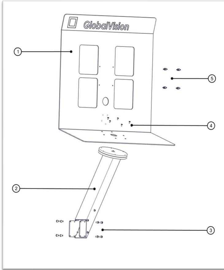
**Figure 2: Swivel Monitor Arm Assembly Parts**
