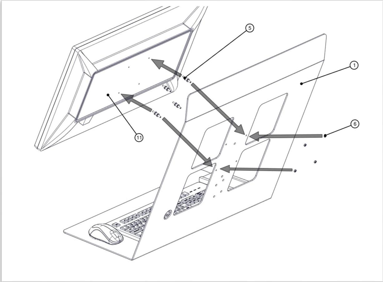
**Figure 6: Attach Monitor Mounting Spacers**
