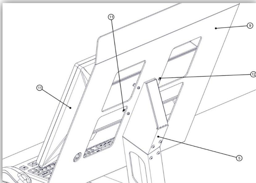
**Figure 8: Attach Monitor to Monitor Plate 2**
