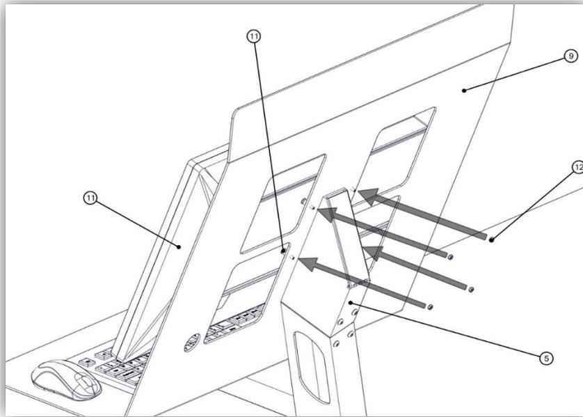
**Figure 7: Attach Monitor to Monitor Plate 1**
