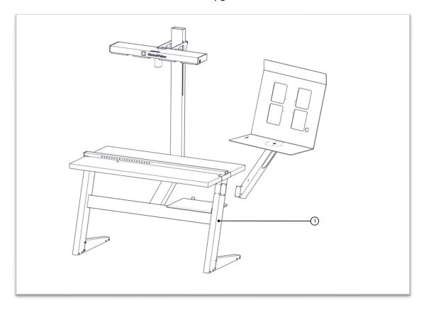
Figure 24: Connecting the monitor arm with the right leg(Part 1)
