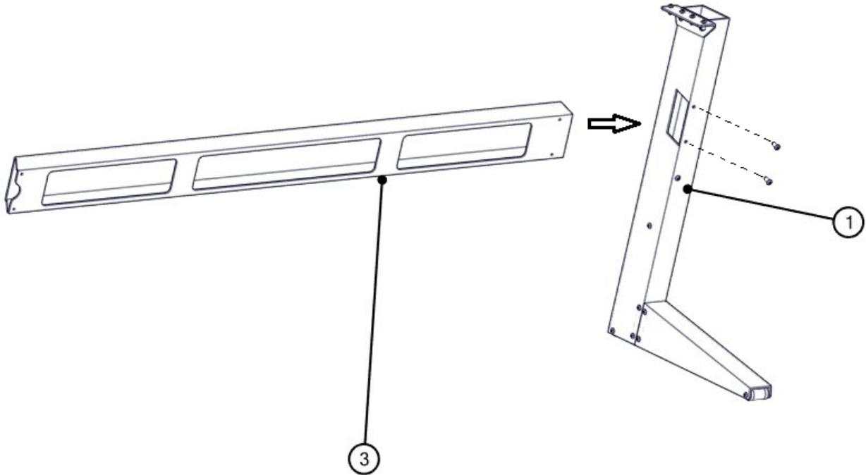
**Step 2:** Connect right leg assembly (Part #2) to horizontal support bar (Part #3) and attach with 2 bolts.
