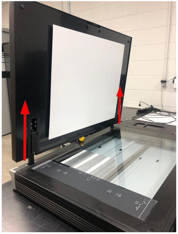
3: Place the lid on a table overhanging the Hinge section as per the image below. This will provide a working room to replace the hinges.
