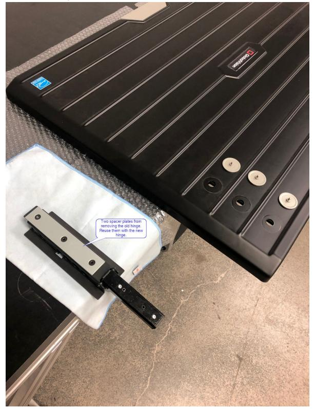
6: The image below shows the bottom of the lid with the hinge removed.
