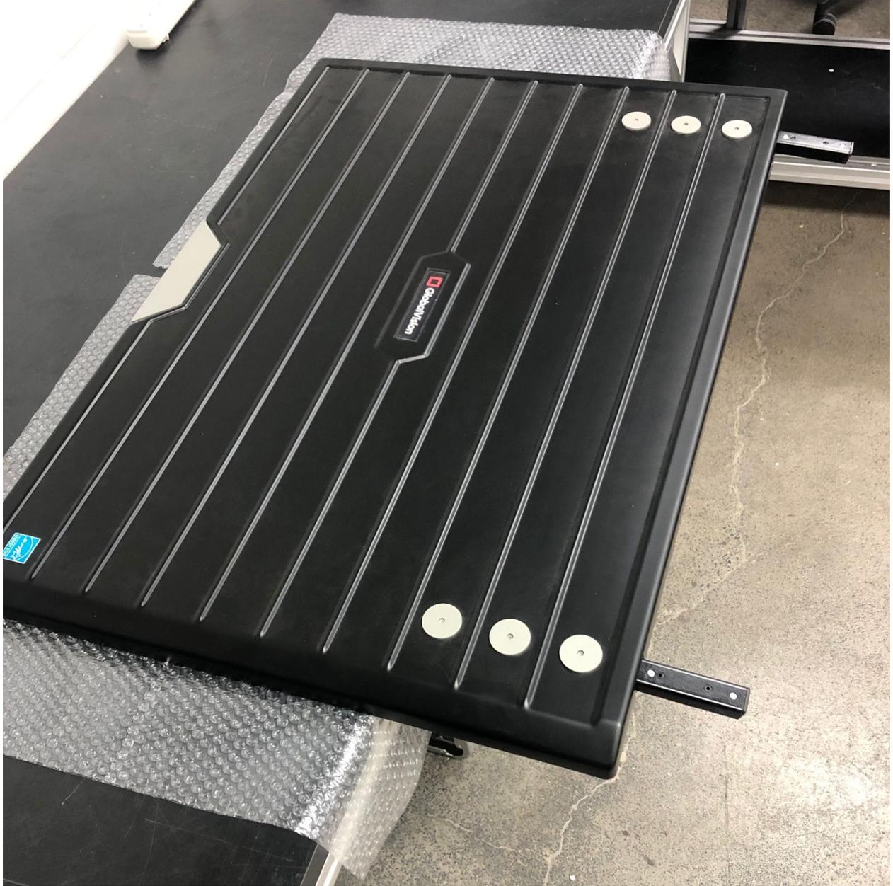
4: Next, Using a 5 mm Allen key tool. Remove the three grey Allen key bolts on top of the lid. Hold the hinge from below, to prevent the hinge from falling down.
