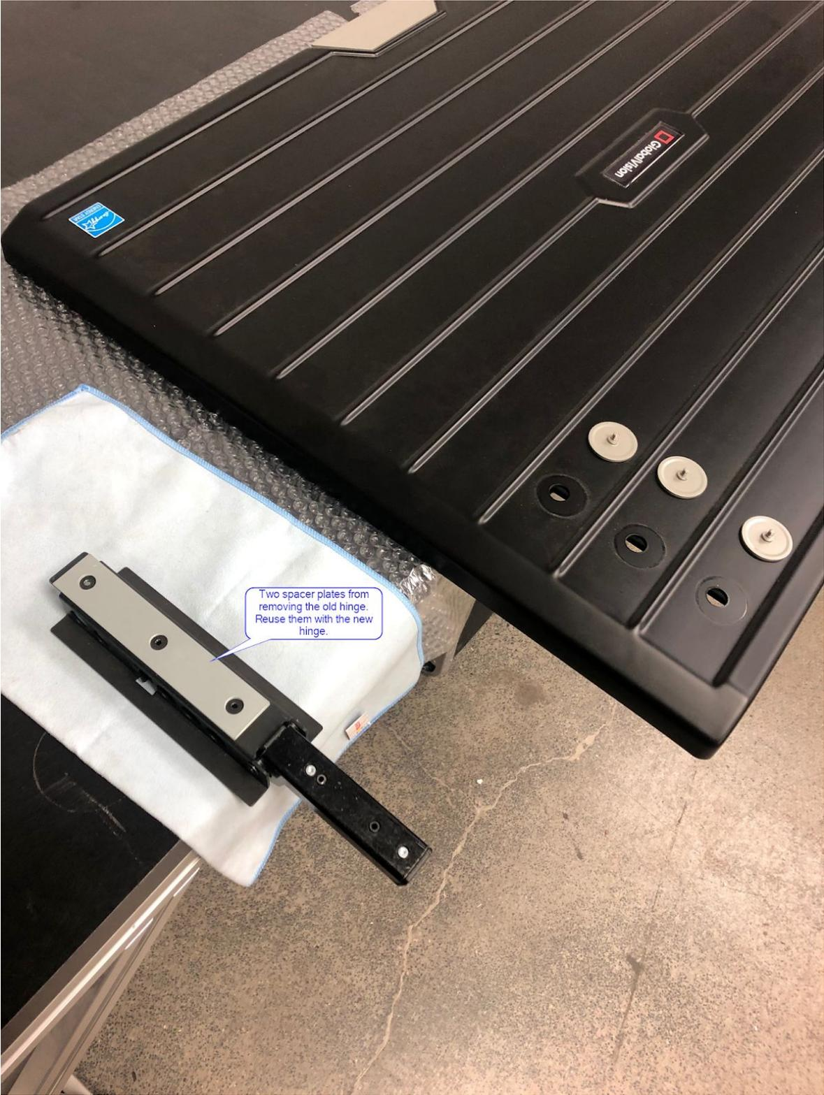
6: The image below shows the bottom of the lid with the hinge removed.
