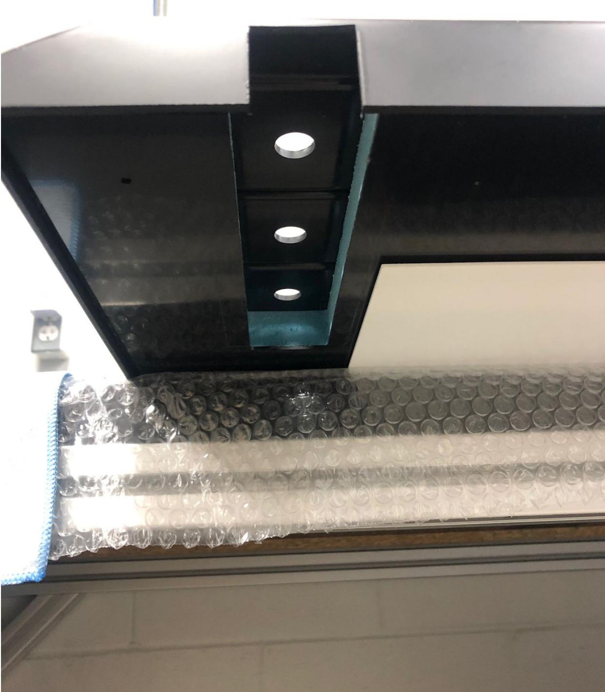
7 : While holding the hinge from below, fasten the three Allen Key bolts onto the previous positions of the Allen Key bolts before tightening them. This will ensure that the lid alignment will not change with the new hinge installations. Do not overtighten the bolts.
