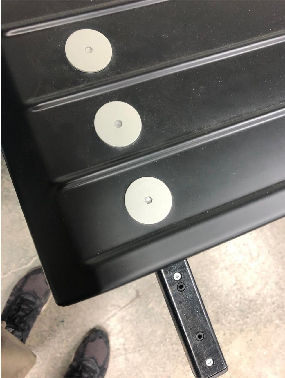
9: Reinstall the scanner lid onto the scanner. Slide the left and right hinges into the two allotted hinge slots on the scanner. See the below image.
